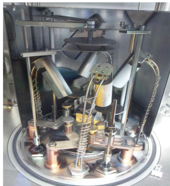
Figure 36 – MBRAUN thermal evaporator and operation principle
